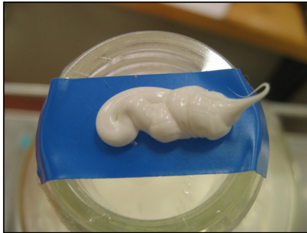
Figure 5.1: Cling wrap, electrical tape and kitchen/bathroom silicone covering the top of a 2 L bottle, through which manual sampling is undertaken with a needle for electronic nose analysis.
